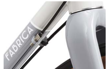
1x11 cable routing
